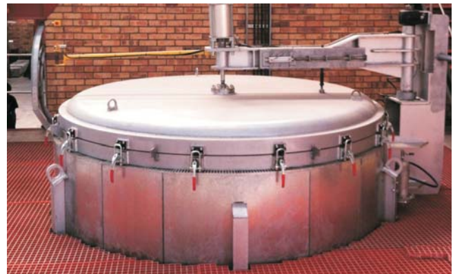
Vacuum Oven - SCADA controlled and monitored.
